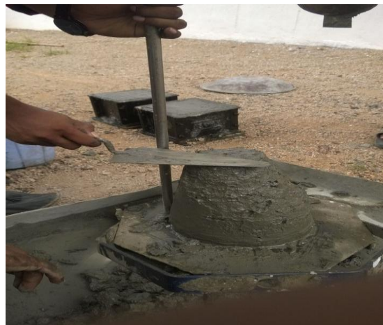
Fig 3: Slump cone test
